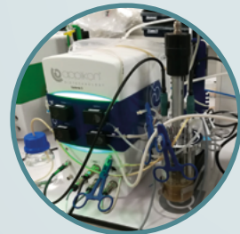
In vitro model of piglet gut (INRA-UCA)
